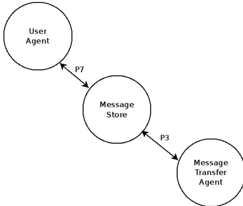
In the CCITT model for implementation of a Message Store, only one protocol is used for communication between the UA and the Message Store - the P7 protocol.
