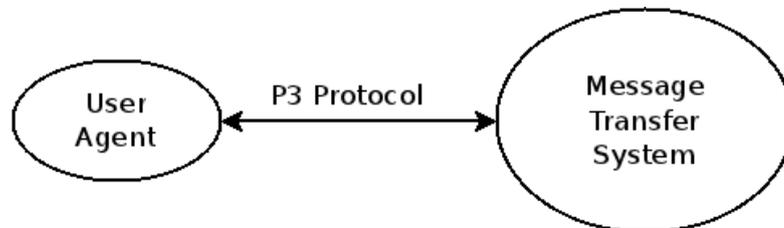
In the basic CCITT model, both inbound and outbound messages are transferred using the P3 protocol. However, the actual protocol used is dependent on the message handling system that is in place and whether or not the MTA and the UA are co-resident.
