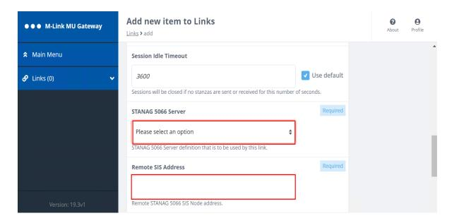
From "STANAG 5066 Server" select 5066-node1. "Remote SIS Address enter the IP address of the remote STANAG 5066 SIS Node Address
