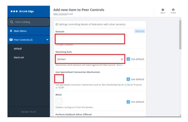
The "Domain" should be the XMPP Domain of the Server you are connecting to. The "Matching Rule" should be "Domain and Subdomain" if you want to include both the 1 to 1 Domain and Multi User Chat (MUC) Domain. You should then select the "Link" you have just created from the drop down.
