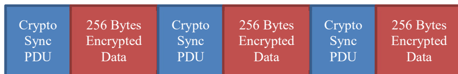
Figure T-7: Crypto Sync PDU repetition for first 4096 bytes of Data
