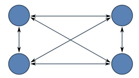
In a standard XMPP configuration, XMPP servers are fully interconnected, as shown in Figure 4.1, "Standard XMPP Server Configuration". This model works well for open XMPP deployments on the Internet. However, it does not work so well for cross domain, organizational boundary and constrained link scenarios.
