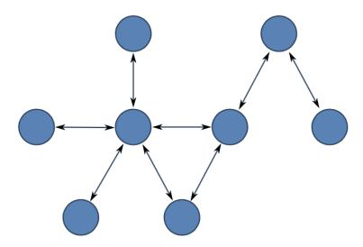
The model of XMPP Trunking, shown in Figure 4.2, "XMPP Trunking" extends the standard XMPP model to allow for configurations where servers are not fully connected. This structure enables XMPP messages to be switched through intermediate servers.
