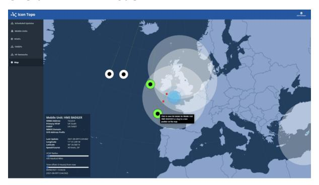
The BRE1TA Model is illustrated by a screenshot from Isode's Icon-Topo product. On the ground, there are multiple HF Access Points (HFAPs). Mobile Units (MUs) will communicate with an HFAP that provides a good-quality HF link. A BRE1TA system requirement is to provide the best HF communication to each MU and to optimize load sharing between HFAPs. This is achieved by assigning MUs to HFAPs with scheduled transfers between HFAPs.
